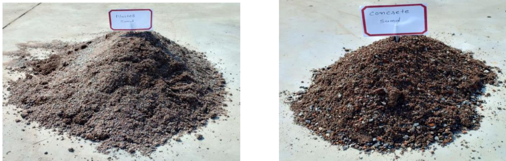
Figure 13. Collected Sample of Plaster Sand and Concrete Sand
